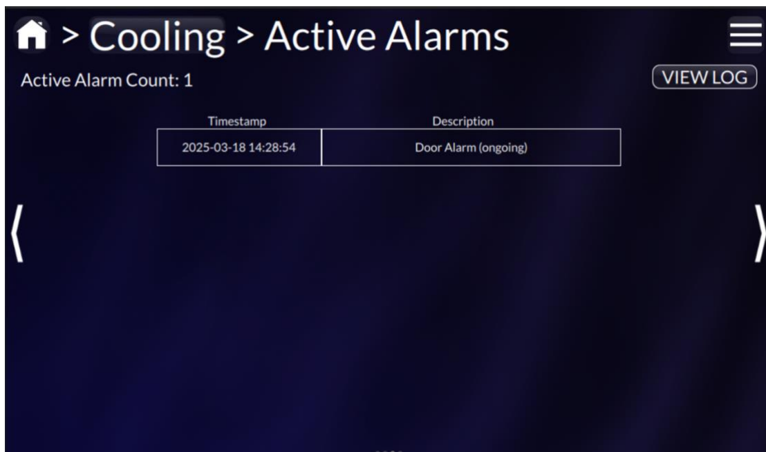
Figure 5-6 Active Alarms Screen (with Active Alarm)
