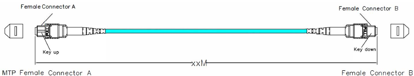
Figure 1 -MTP-MTP 24F Multimode OM4 Fiber Optic Cable
