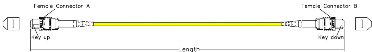
Figure 1 -MPO-MPO 24F Singlemode Fiber Optic Cable
