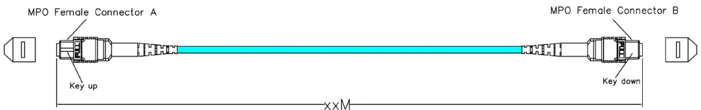
Figure 1 -MPO-MPO 24F Multimode OM4 Fiber Optic Cable
