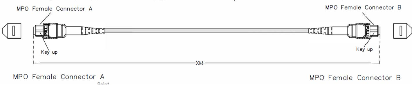
Figure 1 -MPO-MPO 8F Multimode OM4 Fiber Optic Cable
