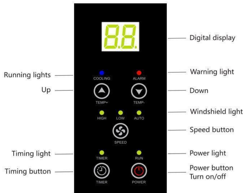
Figure 4.1-1: RCU Controller Interface
