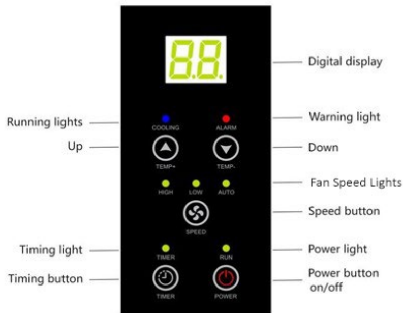
Figure 4.2-1: RCU Controller Interface
