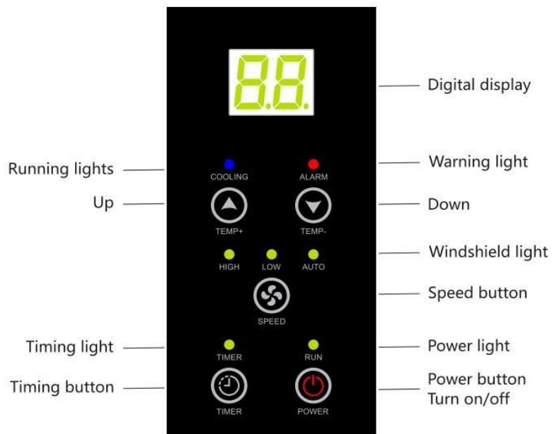
Figure 4.2-1: RCU Controller - Operation Instructions
