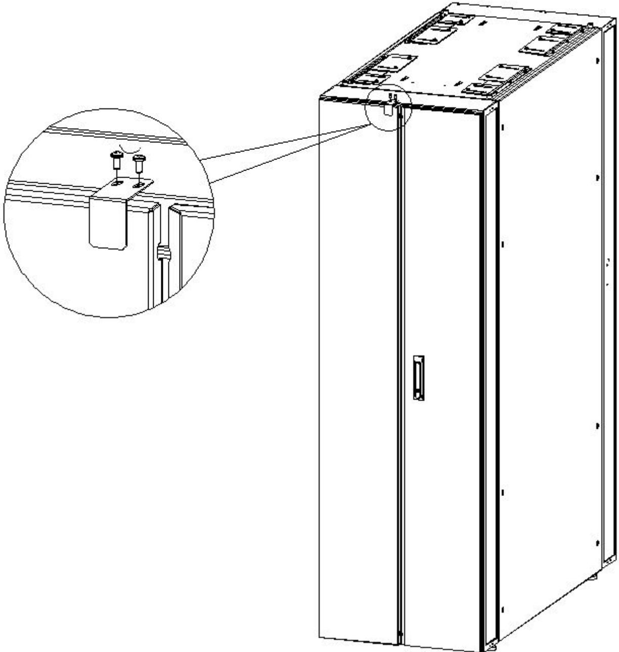
*Figure 7.2-1: Remove the rear fixed door kit*
