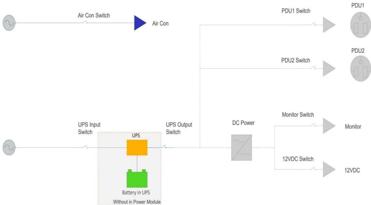
Figure 7.4.2: Electrical Schematic
