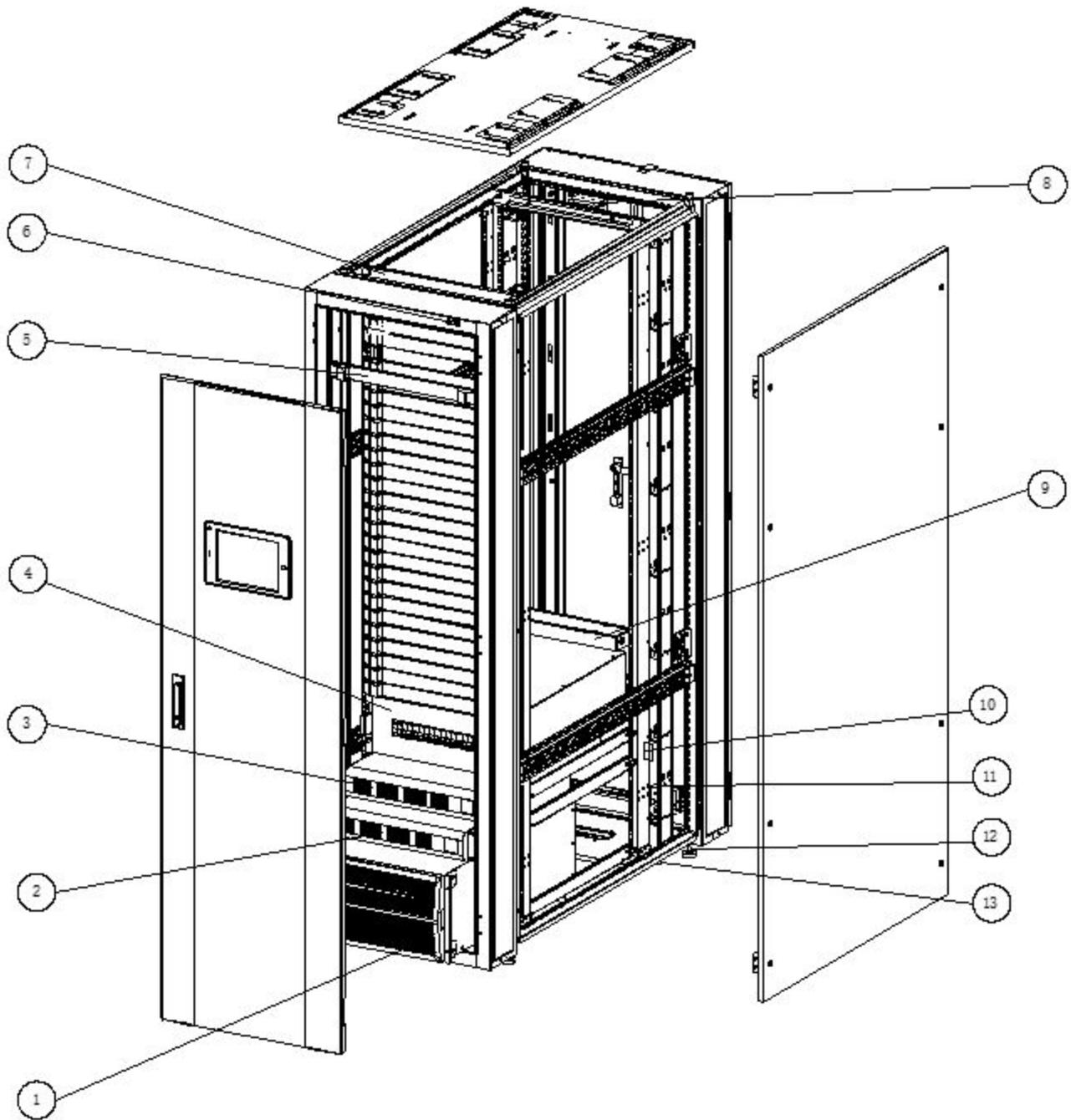
Figure 2-2: EdgeRack 3P Series Interior Components
