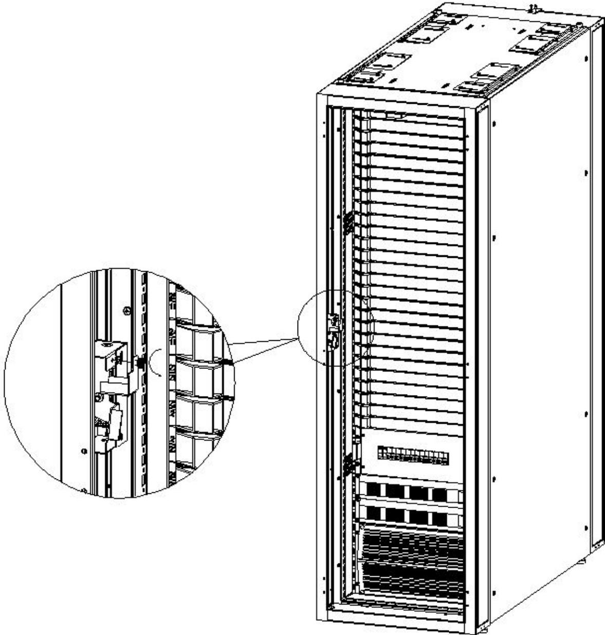
*Figure 7.2-2: Remove the fixed front door kit*
