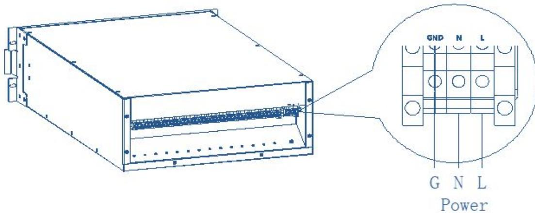
Figure 7.4-1: 32A Rack Mounted Distribution Unit
