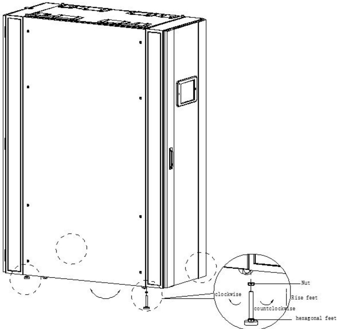
*Figure 7.3-1: Leveling Cabinet & Air Conditioning Unit*
