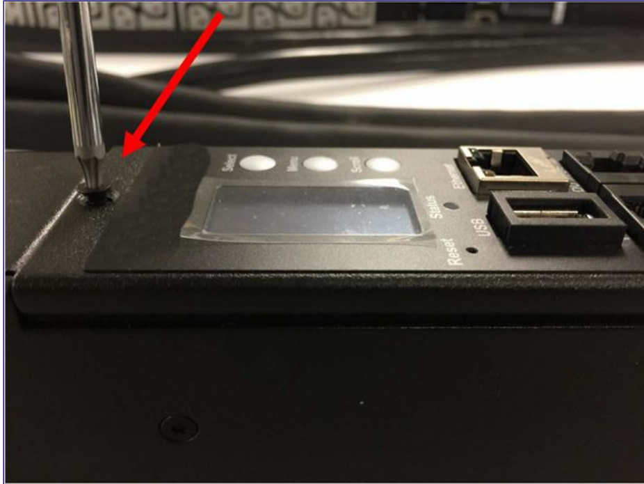
Appendix F Figure 1: Removing Top and Bottom Screw from Intelligent Network Controller
